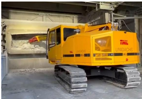
Unidachs 535 - Tundish cleaning
